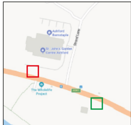
Site D. 40mph A361 Ashford to Braunton ASC Sector by St Johns Garden Centre at Ashford. New ASC sector entrance and exit cameras located separately. These will replace two existing spot speed GATSO speed cameras.
